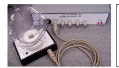
Connect the transducer interface (EIPF) to the main unit using the 8 pin mini DIN cable
