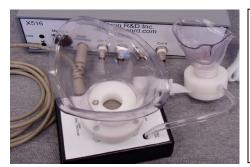
Connect the nasal mask to the transducer interface channel 3 (nasal flow) using nylon tubing.
